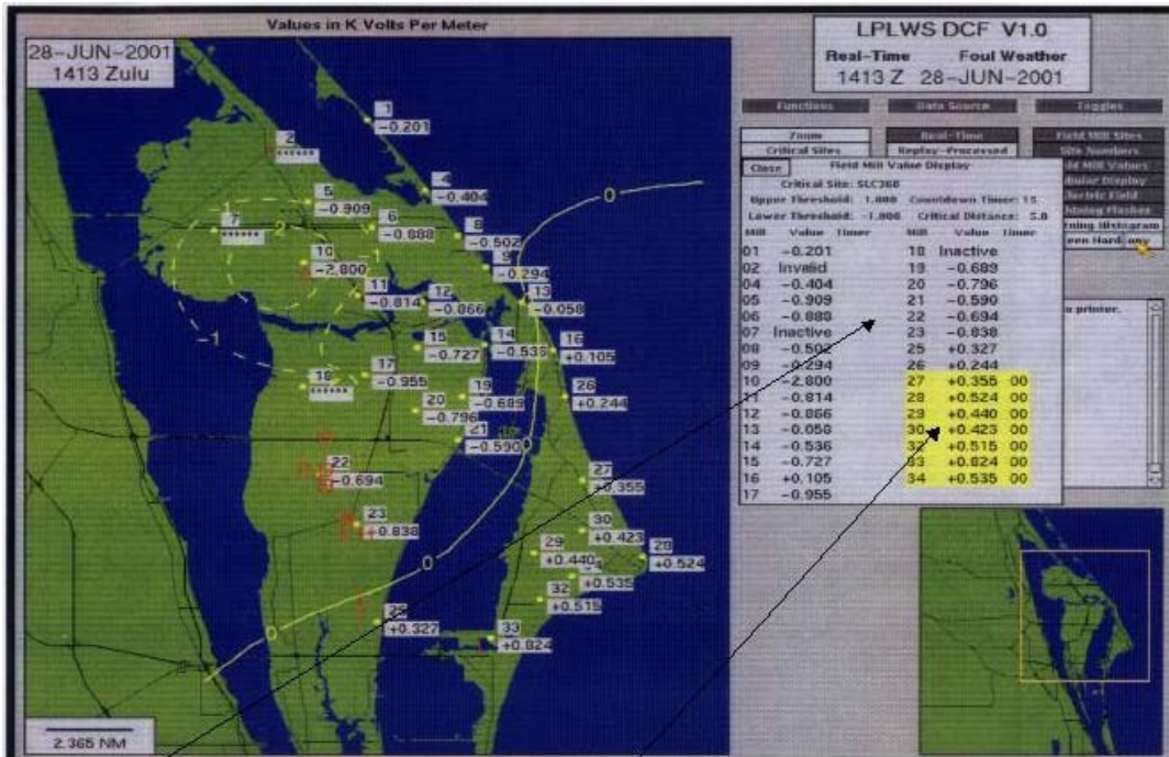
Tabular data: Field mills with 5nm of Complex are hi-lited in Yellow. Non-violated.
